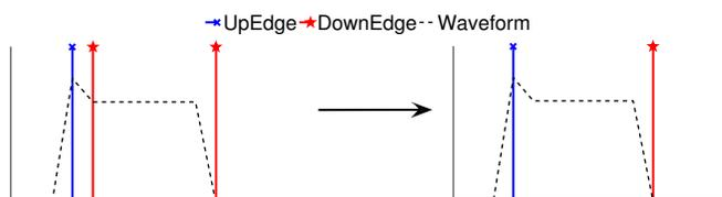
Fig. 9: Noisy Edge caused by a jitter
