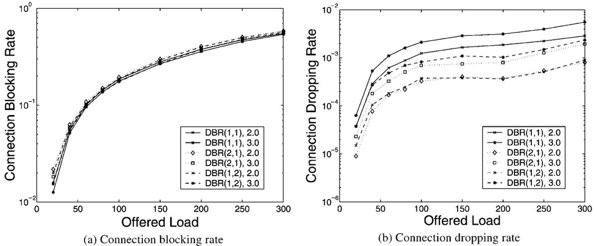
Fig. 10. CBR and CDR of DBR approach with different sector configurations and sharing rates ( $\epsilon = 1.5$  and  $\eta = 2.0$  or  $3.0$ ).
