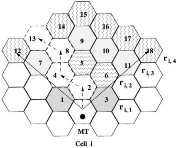
Fig. 3. An example of the user profile-based differential bandwidth reservation (UPDBR) policy. For the original DBR policy, all the cells starting from  $c_1$  to  $c_{18}$  may participate in bandwidth reservation. Whereas in the UPDBR approach, only cells  $c_2, c_4, c_8$  and  $c_{13}$  are involved in the bandwidth reservation.
