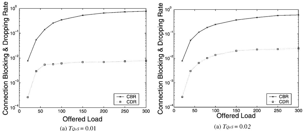
Fig. 6. Connection blocking and dropping rate with different  $T_{QoS}$  ( $\epsilon = 1.5$  and  $\eta = 3.0$ ).
