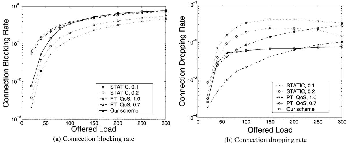
Fig. 5. Comparisons of the Connection blocking rate (CBR) and Connection dropping rate (CDR) of the proposed scheme ( $\epsilon = 1.5$  and  $\eta = 3.0$ ) with the STATIC scheme ( $g = 0.1, 0.2$ ) and the PT-QoS scheme ( $S = 1.0, 0.7$ ).
