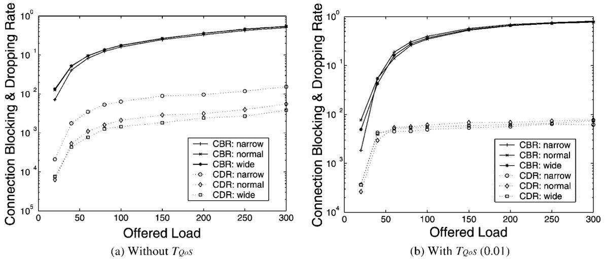
Fig. 12. Connection blocking and dropping rate with different number of cells in each cluster.
