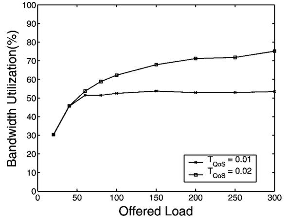
Fig. 7. Bandwidth utilization with different  $T_{QoS}$  (0.01 and 0.02).
