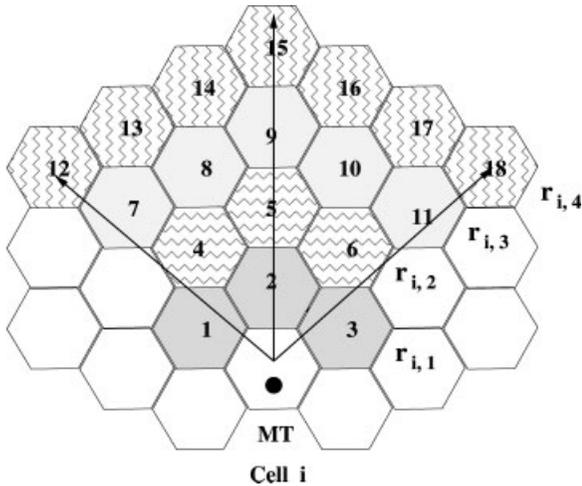
Fig. 1. Classification of sector of cells into different clusters based on their distance from the current cell.
