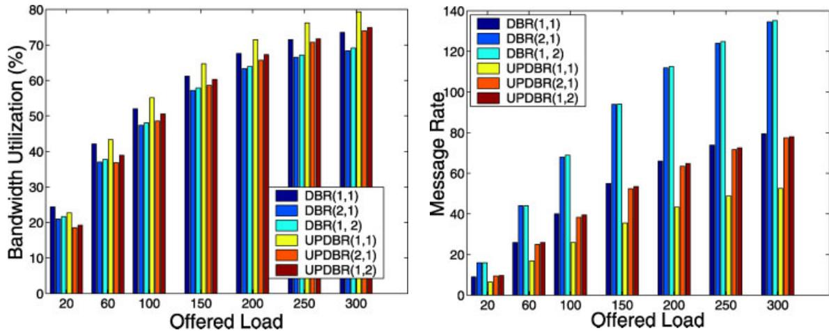
Fig. 14. Comparisons of the UPDBR approach to the DBR approach ( $\epsilon = 1.5$  and  $\eta = 2.0$ ). Six bars for different policies and sector configurations are shown against offered load. The DBR(1,1), DBR(2,1), DBR(1,2), UPDBR(1,1), UPDBR(2,1) and UPDBR(1,2) schemes are plotted from left to right.
