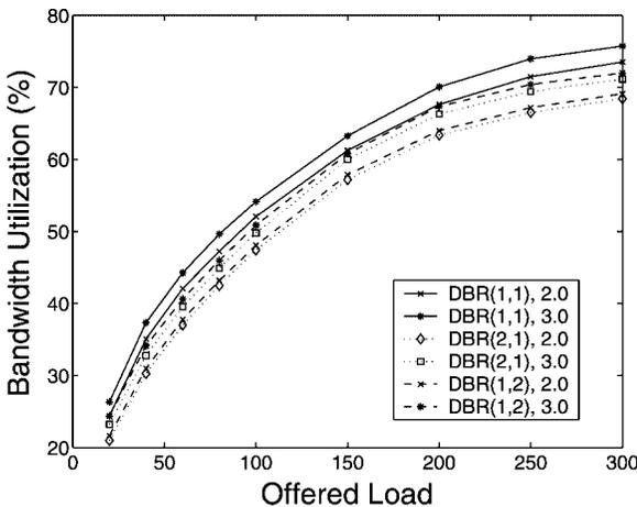
Fig. 11. Bandwidth utilization of DBR approach with different sector configurations and sharing rates ( $\epsilon = 1.5$  and  $\eta = 2.0$  or  $3.0$ ).
