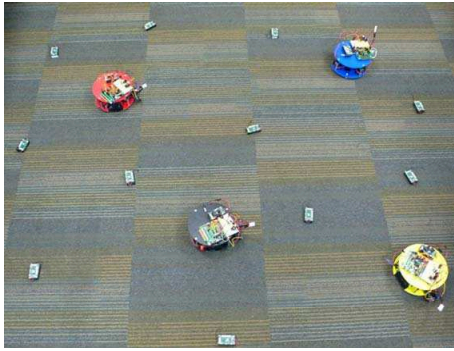
Fig. 3. The prototype which consists of mobile sensors and static sensors
