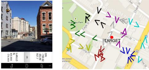
Fig. 2. (a) Screenshot of the programmed phone. (b) We take 40 photos and assign them to 8 nodes in the trace. The locations and orientations of the photos are shown in V shapes, where the photos assigned to different nodes have different colors.
